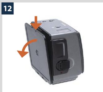
1. Remove the battery holder from the grip by depressing the battery holder button and simultaneously swinging the battery holder retaining lever down until it stops. Pull battery holder downwards.
