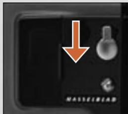
To raise the flash unit into its operative position, slide the flash-unit catch backwards in the direction of the flash symbol. To return the flash unit into its closed position, push down on the top of the unit until it clicks back into place. The flash unit is automatically activated when it is in the operative position and de-activated when returned to its stored position.
