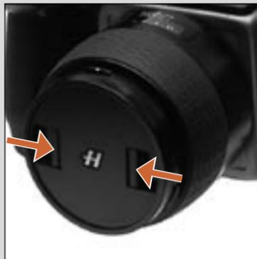
by unscrewing it in a counter-clockwise direction. Align the index on the lens with the index on the camera body and rotate the lens clockwise (bayonet fitting) until it clicks into place.
